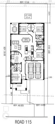
(A EASEMENT TO DRAIN WATER 1.5, 2 WIDE AND VARIABLE WIDTH (B) EASEMENT FOR SUPPORT 0.5 WIDE (C) EASEMENT FOR MAINTENANCE AND REPAIRS 0.9m WIDE BASIX 90 INCLUDING 6.6 KW SOLAR
